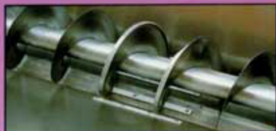
Coclea senza supporto intermedio Screw feeder without intermediate support Vis sans fin sans support intermédiaire
